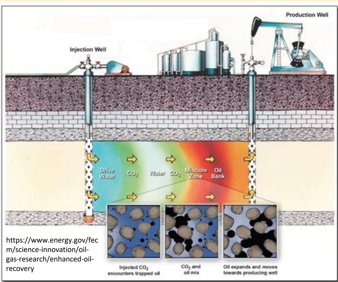
During the EOR (WAG (Water Alternating Gas) (HC gas) or CO<sub>2</sub>)
